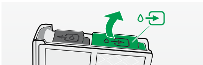
Fig. 3.5 Opening the fresh water tank
