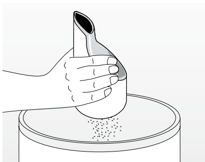
Fig. 4.3 Emptying the dust chamber
