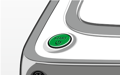
Figure 3.17 Press the start/stop button on the Robot Vacuum Cleaner for standby mode.
